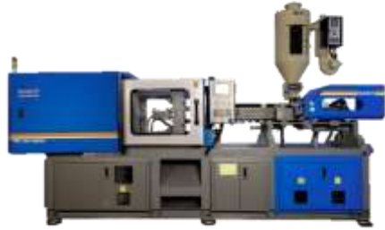
PLASTIC INJECTION MACHINES
